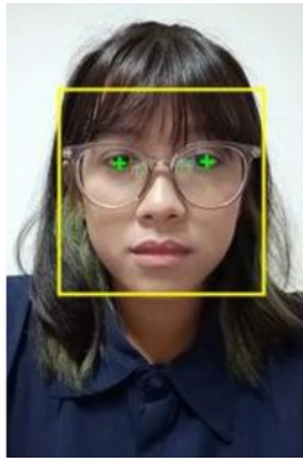
Figure 3 Face and pupil identification in a particular frame
